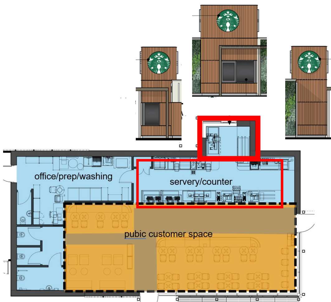
figure 43: Tower location over the kitchen area
